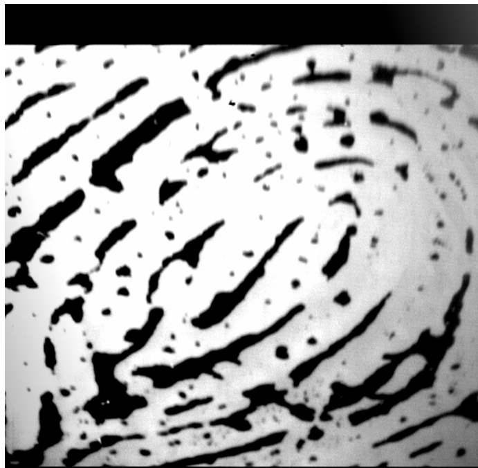
High pressure – only the largest of the edge features are obvious – most of the detail has been obliterated.
